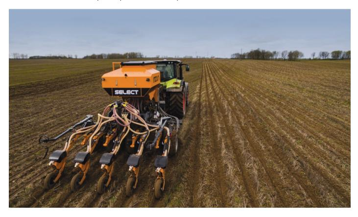
Marking a huge advance in seeding technology, the innovative Mzuri Pro-Til Xzact combines a striptill drill and a precision seeder in just one piece of equipment, meaning that one drill can now seed all types of arable and precision crops – in a single pass.
