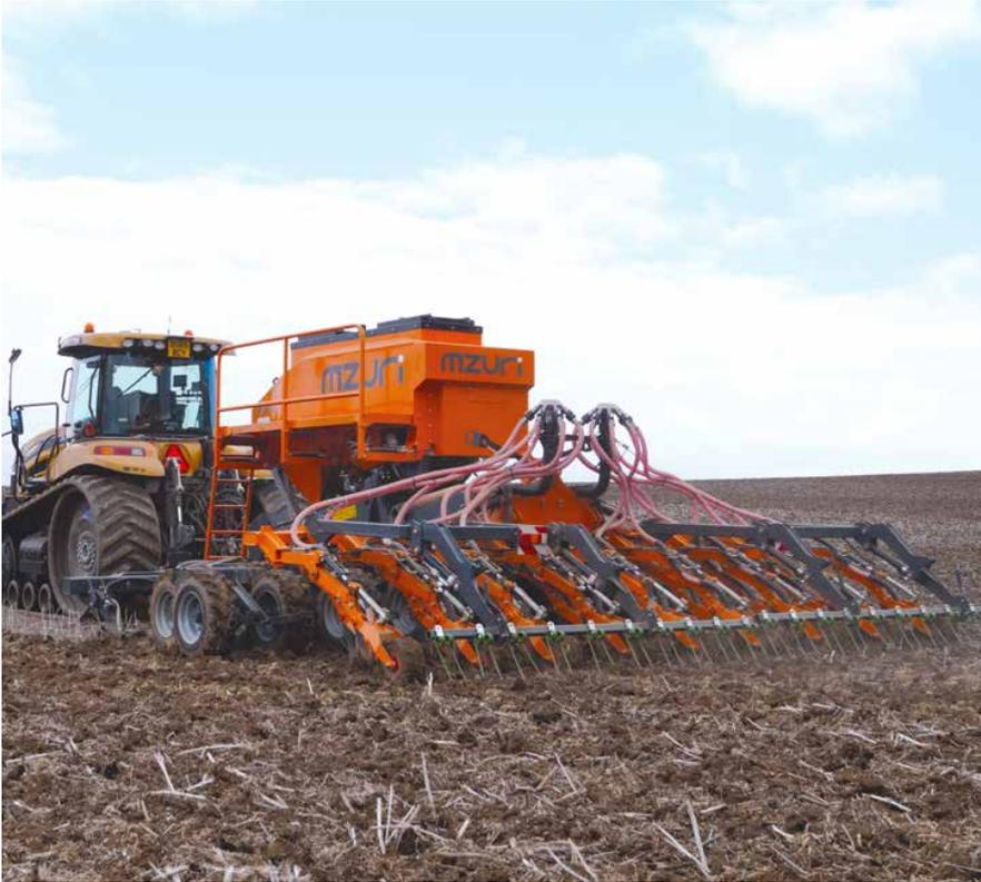
As well as all the benefits of a standard Mzuri PRO-TIL drill, the Mzuri PRO-TIL Select series can drill in a choice of narrower or wider row spacings. The wide row option makes the Select particularly suited for crops such as maize, oilseed rape and legumes. It is equally at home with drilling narrowly-spaced crops including wheat, barley and oats.
