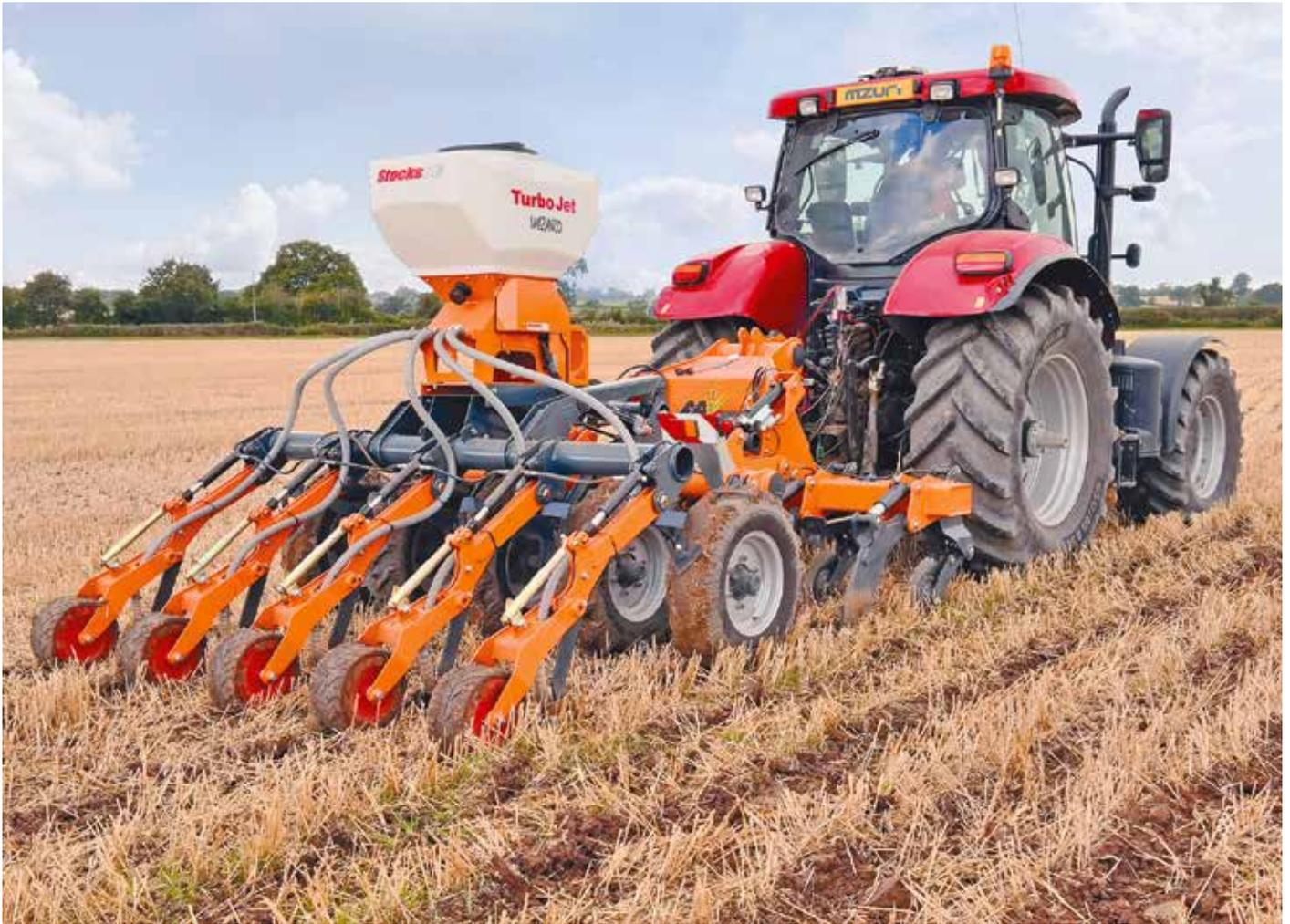
The REHAB subsoiler is available with an option of a seeder unit – ideal for drilling oil seed rape and cover crops. The individual coulters give an accurate sowing depth into a friable seedbed; this provides the ideal soil environment for each seed, ensuring rapid and even germination.
